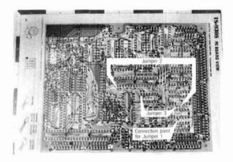
fig. 5. Location of connection points for mod 4.
